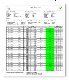
Apply rules to Auto Test and OPM data to ensure fibers meet required specifications. Pass/Fail indication for each test simplifies the review of test results.
